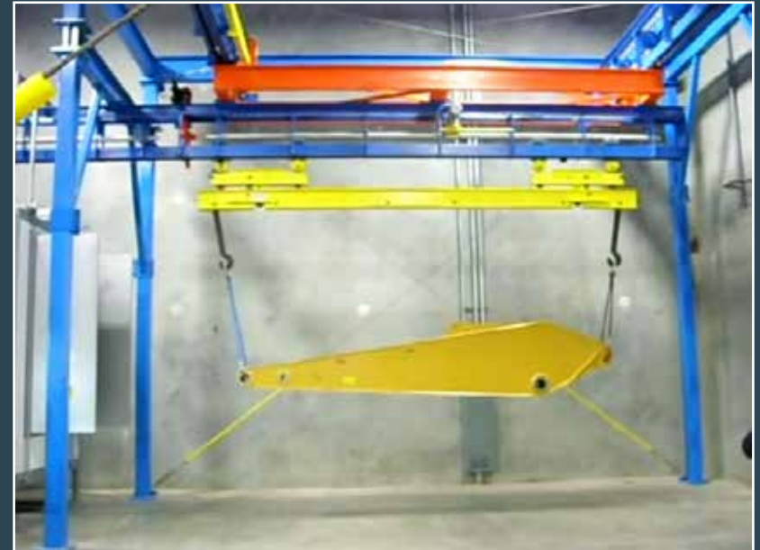
Space saving shuttle eliminates need for large radius turns
