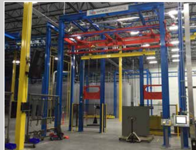
Lifts are frequently used for IntelliFinishing systems for ergonomic loading and unloading of parts
