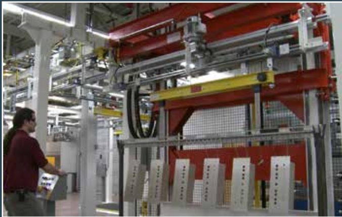
The lift provides efficient, safe and ergonomic loading and unloading of parts
