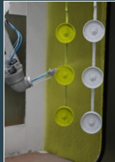
*Robotic paint application is programmable for part specifications & requirements and provides a consistent, quality finish to every part*
