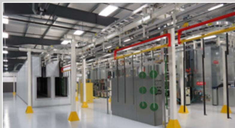
*Dual-lane cure oven allows parts of different sizes move at different speeds during the curing process*
