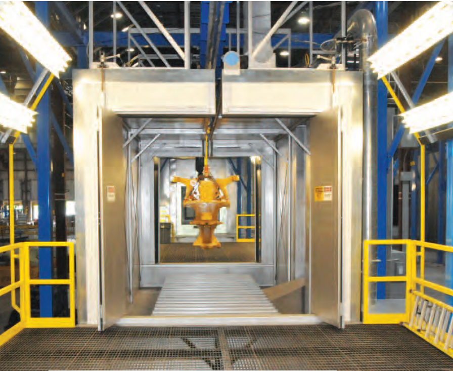
Dry-off oven doors open as parts proceed from the blow-off deck through the oven on to the mask deck.
