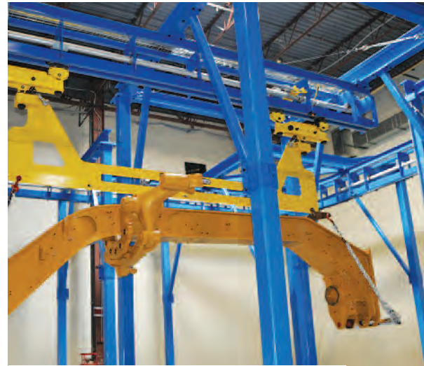
Spurs throughout the system allow for parts to be pulled offline and re-entered into the system.
